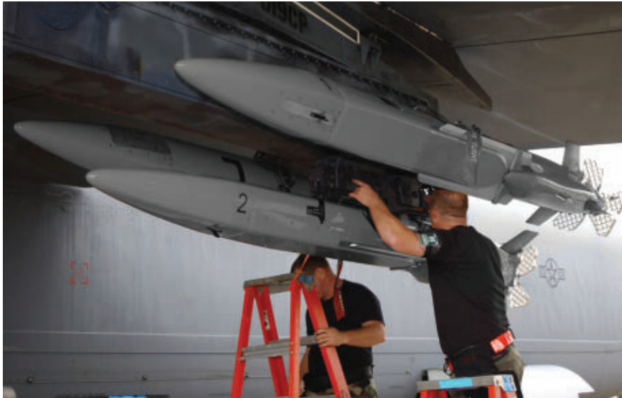
The Raytheon Miniature Air Launched Decoy Jammer (MALD-J), shown above, is a relatively simple air-launched unmanned aerial vehicle (UAV) designed to jam and spoof enemy radar.
