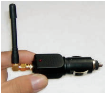
Small jammers that disrupt GPS signals are available at low cost that can fit in a car's cigarette lighter.
