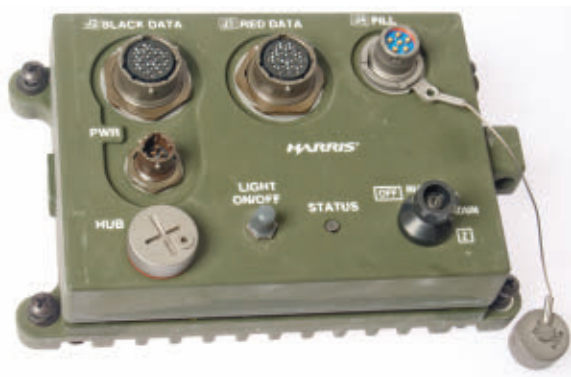
The Harris Corp. RF Communications segment in Rochester, N.Y., designs and manufactures the KGV-72 encryption device, shown above, which provides the ability to process classified messaging traffic.
